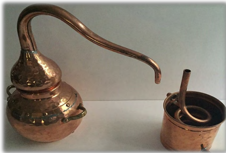
Alembic still showing column decoupled from the condenser:
