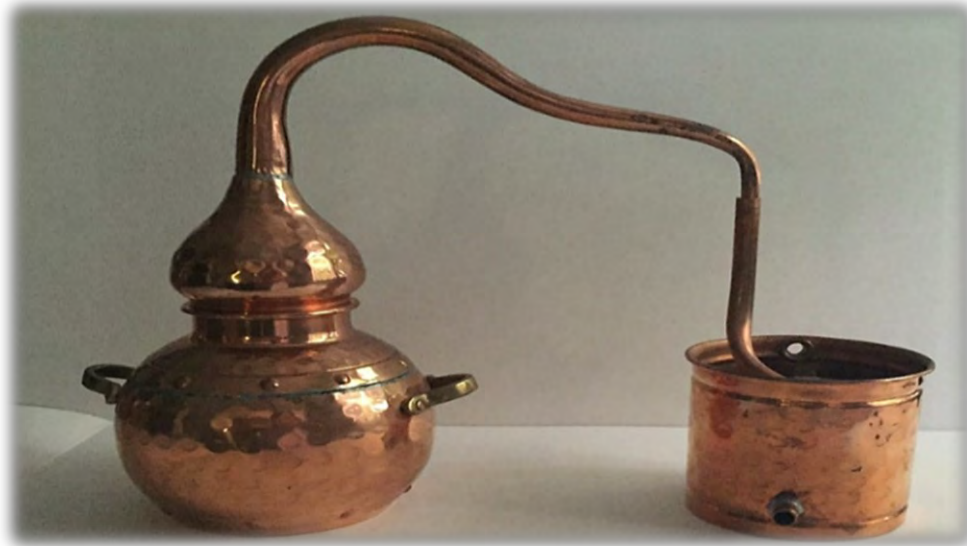
Alembic still showing column decoupled from the condenser:
